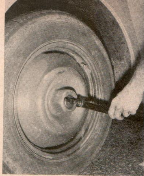
The actual work of removing the wheels is still for the owner, but it's not too rugged with only one lug bolt
